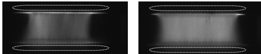
Fig. 5 ICCD camera images of a nanosecond pulsed discharge in nitrogen at P_0 = 350 torr. Pulse-repetition rate \nu = 100 kHz. Pulses 100 (left) and 1000 (right).
